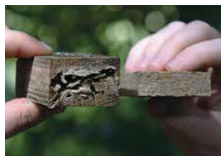
Untreated wood (left), LP SmartSide (right)
