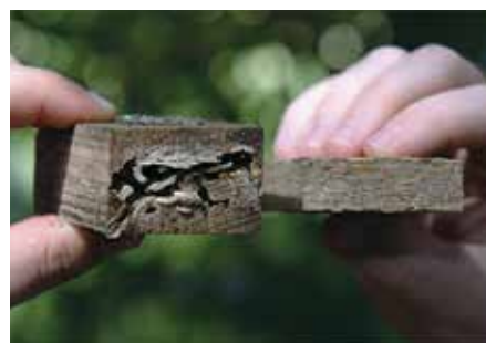
Untreated wood (left), LP SmartSide (right)
